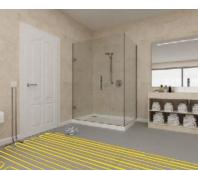
Prepare floor plan of the area to be heated and identify suitable location of the fused spur and thermostat position - mark the layout of the underfloor heating mat on the floor plan. This is an important step and must be carried out correctly to ensure that all the mat is used up. Once a mat has been unrolled it can not be returned.
